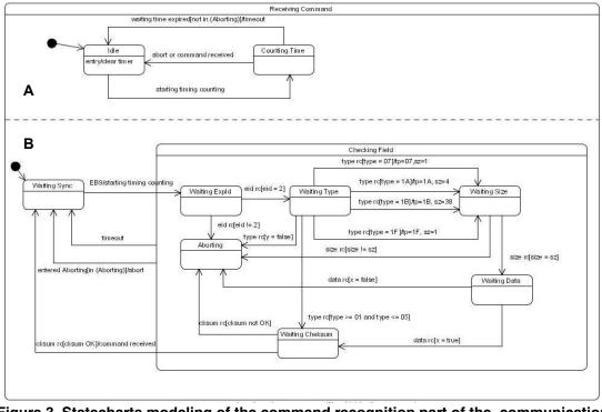
Figure 3. Statecharts modeling of the command recognition part of the communication protocol.
